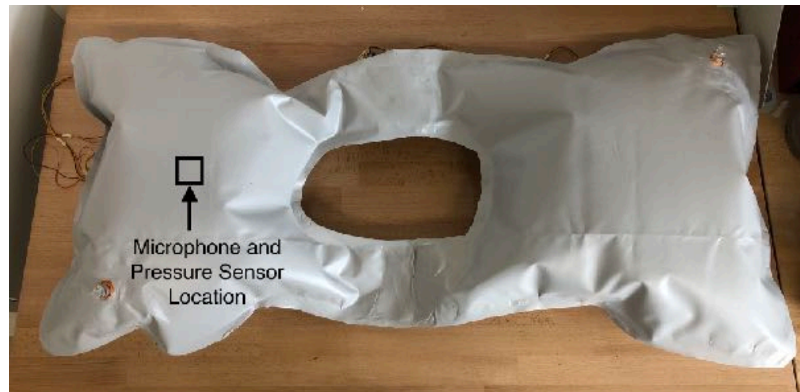
Inflated chest with internal microphone and pressure sensor
